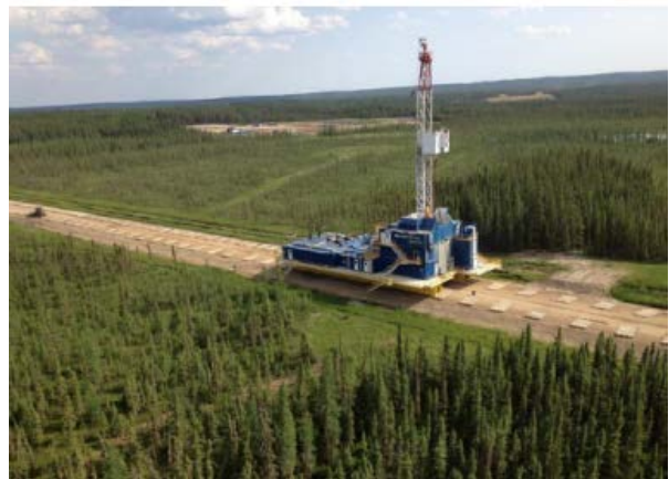
Fully-assembled rig moving between pads
